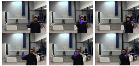
Fig. 4. Hand being tracked by the Gest module : the ellipses are the projection of the 3D state vector
