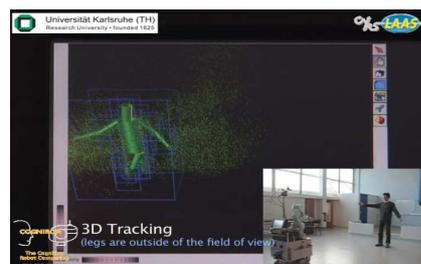
Fig. 7. The Voodoo module interface (background) showing the 3D body model estimated configuration with respect to the real scene (bottom right).
