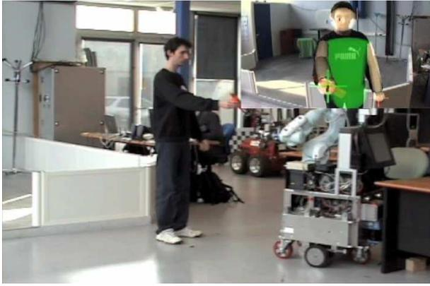
Fig. 1. A typical situation of Human-Robot interaction. The upper right part of the image represents the robot perception and the superimposed avatar is the estimated configuration.
