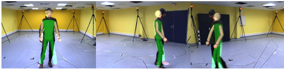
Fig. 10. Images from the three cameras with avatar reprojection taken during the walking sequence, which presents partial occlusions of body members.
