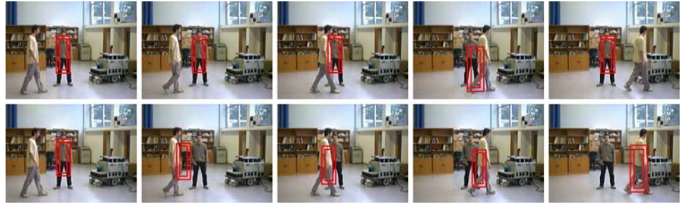
Fig. 35 Tracking scenario involving occlusion of the motionless target by another person crossing the field of view with DMIF-RBSSHSSIR (top) and HIERARCHICAL_PF (bottom)
