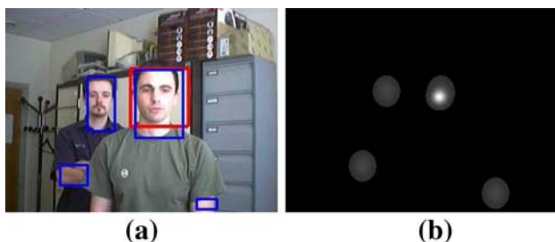
Fig. 11 a Skin blobs (blue) and face (red) detectors. b Importance function mixing their outputs
